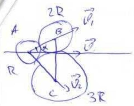
$$\begin{cases} \text{ЗCU: } m\vec{V} = m\vec{V}_1 + m\vec{V}_2, \\ \text{ЗЭЭ: } \frac{mV^2}{2} = \frac{mV_1^2}{2} + \frac{mV_2^2}{2} + Q. \end{cases}$$
